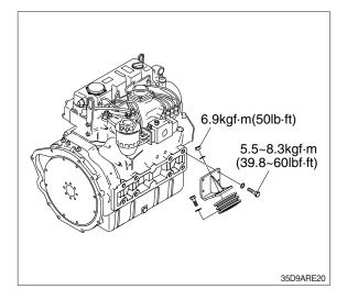
(3) Tightening torque of mounting bolt installing to torque converter housing.
